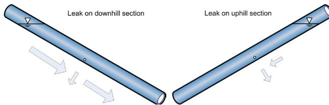
**Figure 3.** Typical leak scenarios on downhill and uphill sections when applying COESD procedures.
