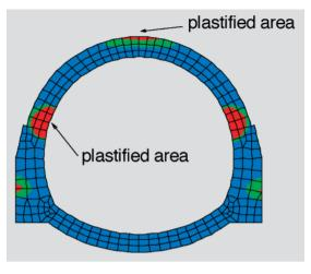
The thickness of the lining in the investigated section amounts to 90 cm in the crown, 120 cm in the benches and 80 cm in the invert (Figure 2).
