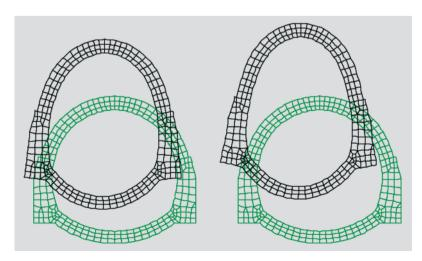
As long as the eccentricity e = M/N is less than d/6 (d = thickness of the lining), compression stresses act in the whole section. In this case no failure is to be expected since the compressive strength is relatively high. In case the eccentricity is more than d/6, tensile stresses act in the lining which cannot be carried by the mortar. The joints between the blocks will open. The tolerable limit according to common practice is an eccentricity which results in an open joint less than d/2.
