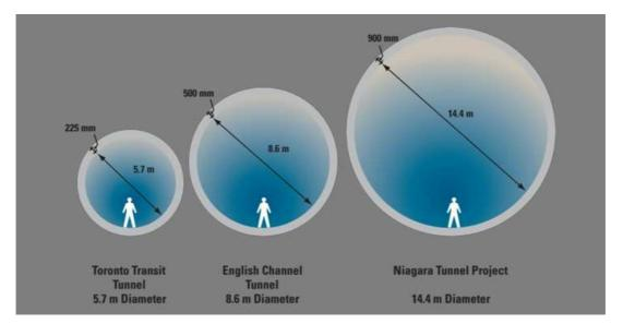
Figure 13: Cross section of the Niagara Tunnel (right) as compared to the cross section of the Toronto Metro (left) and Channel Tunnel (centre).
