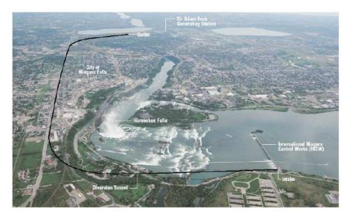
Figure 10: Niagara Tunnel Project: Bird's eye view (Delmar, Charalambu, Gschnitzer, Everdell 2006).
