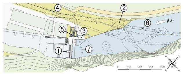
Figure 3: Layout (legend: 1 = KW Hochwuhr; 2 = old intake of the headwater channel; 3 = new intake; 4 = rehabilitated headwater channel; 5 = fish pass; 6 = lateral weir; 7 = "Hochwuhr").
