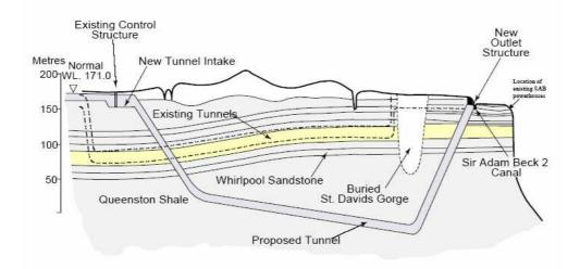
Figure 12: Niagara Tunnel Project: Longitudinal section
