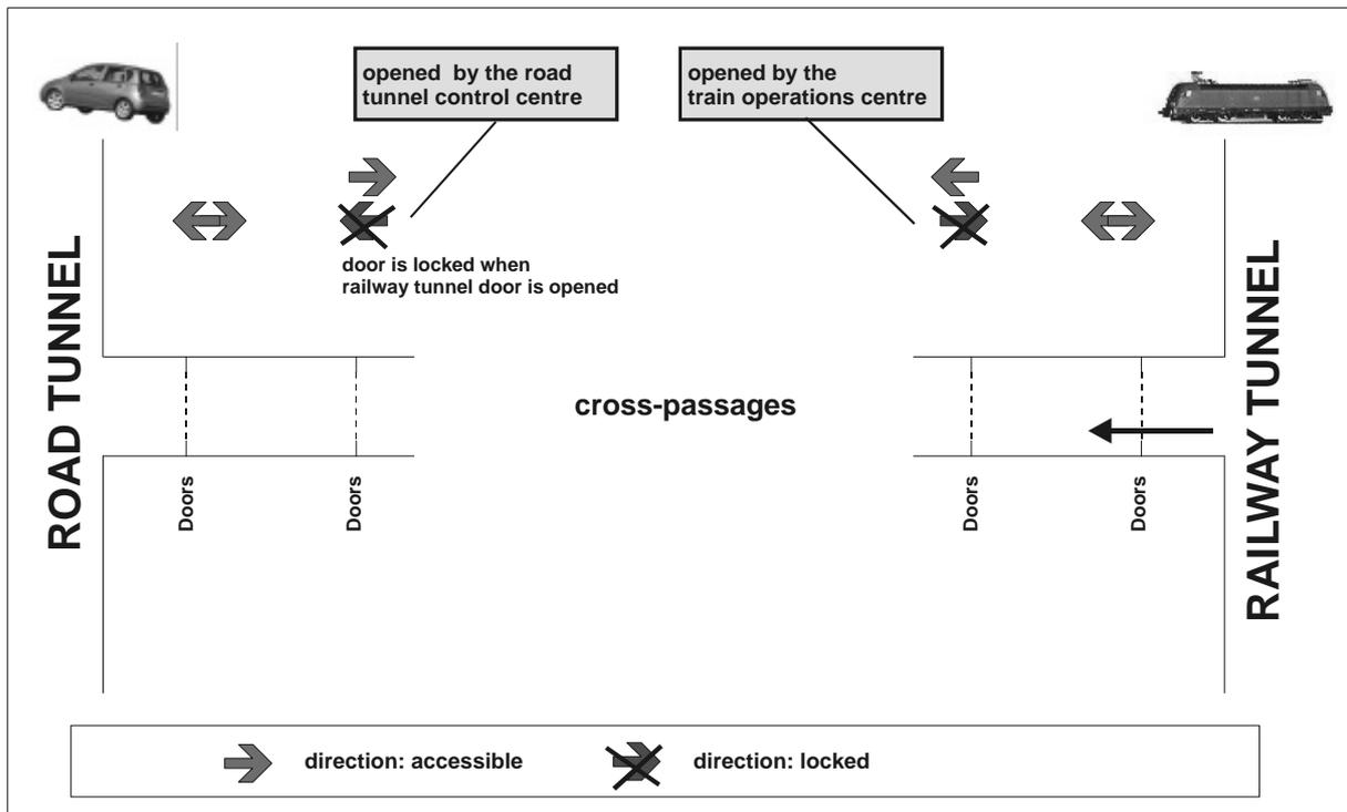
**Fig. 6: Door opening options – accident in railway tunnel**
