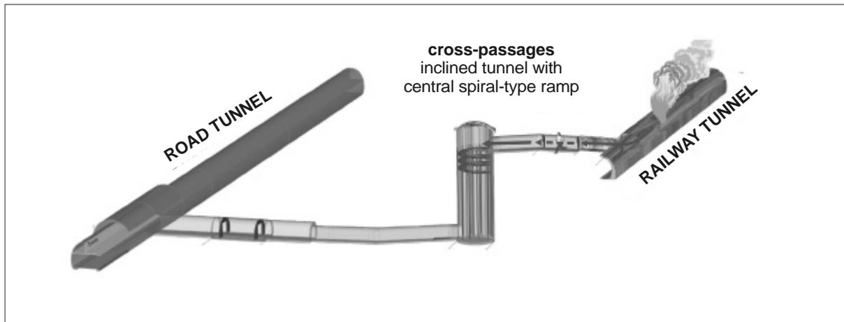
**Fig. 4: Cross-passage with spiral-type ramp**
