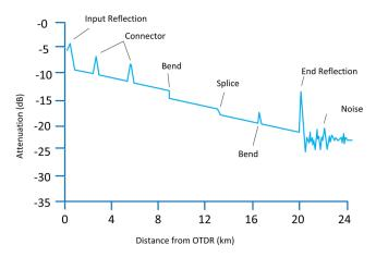
Figure 4. Analysis of fibre losses using OTDR technology.
