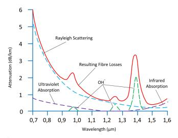
Figure 2. Causes of attenuation in optical fibres.
