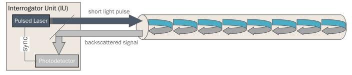
Figure 6. A DAS Interrogator Unit receiving backscattered signals from the fibre.
