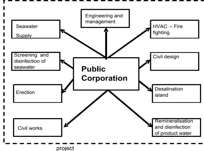
Each of the turnkey contractors is in turn delivering work packages as shown in Figure 7.2 below.
