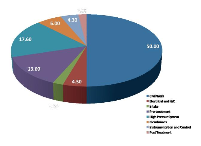
Figure 14.10 : SWRO cost breakdown : alternative case
