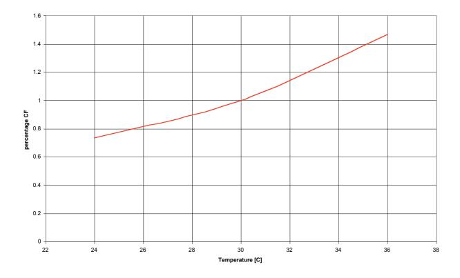
Figure 11.5: variable O&M correction factor against seawater temperature for SWRO technology
