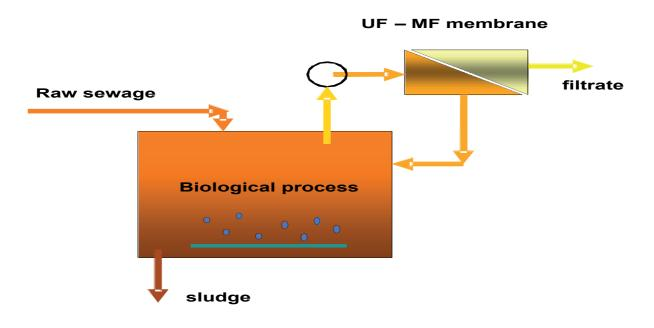
Figure 5.111 side stream waste water pressure system
