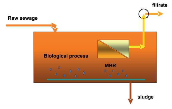
Figure 5.12 vacuum type submerged MBR
