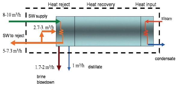
Figure 6.3: seawater requirement MSF process typical flow sheet
