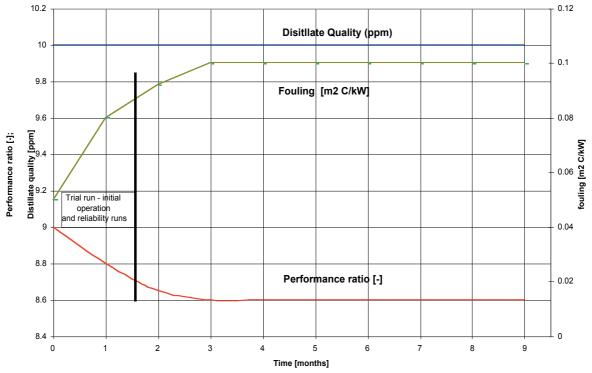
Figure 7.3 Typical MSF performance ratio behaviour between acid cleanings
