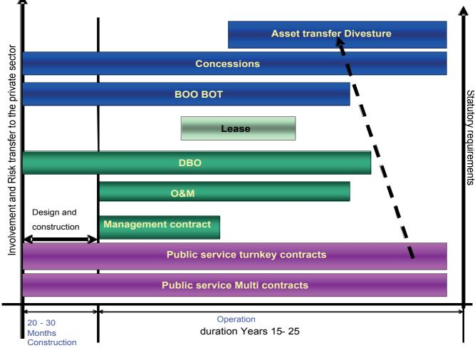
Figure 7-1 desalination plants construction and operation models
