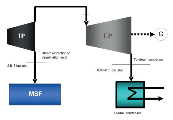
Fig. 6.8 condensing steam turbine feeding an MSF desalination system
