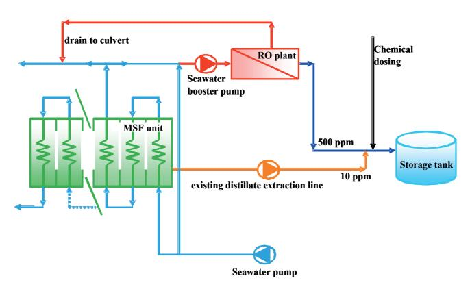
Figure 5.8: Integrated hybrid system flow diagram
