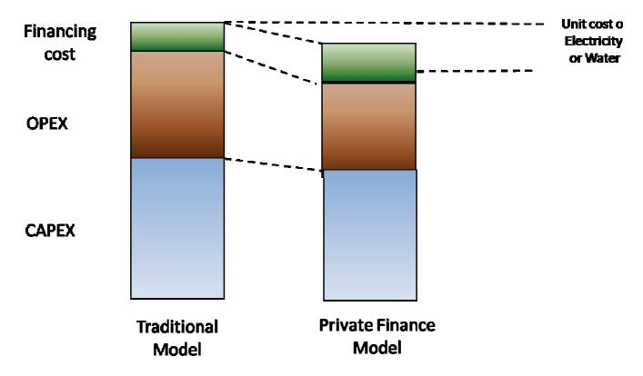
Figure 7.6: traditional turnkey versus private project typical CAPEX OPEX and financing cost structure
