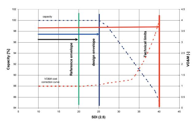
Figure 12.3: reference, design and technical limits envelopes
