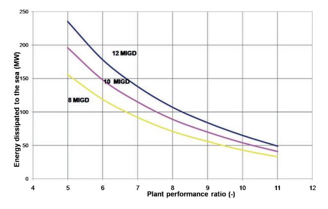
Figure 6.5: energy dissipated with cooling water flow diagram thermal desalination plants
