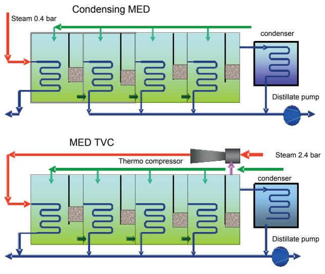
Figure 5.3 condensing MED unit and MED-TVC schematic difference
