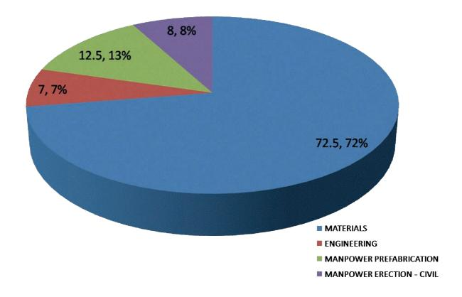
Figure 14.3 : typical cost break down material - manpower for a thermal desalination plant
