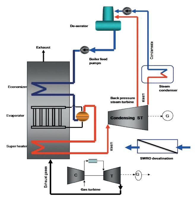
Figure 6.17 Cogeneration scheme with condensing steam turbine and SWRO desalination
