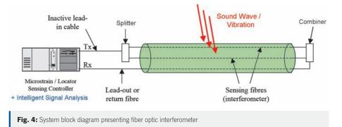
method allows covering large route sections due to simplified cable installation method.
