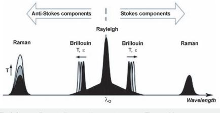
Fig. 2: Scattering effects within fiber optic cables caused by temperature [T] or strain  $[\epsilon]$
