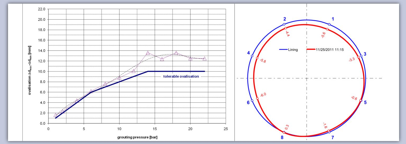
potentially stressed to its limits, its performance needs to be monitored closely during grouting works. The measured deformations are checked constantly against defined permissible ovalisations.
