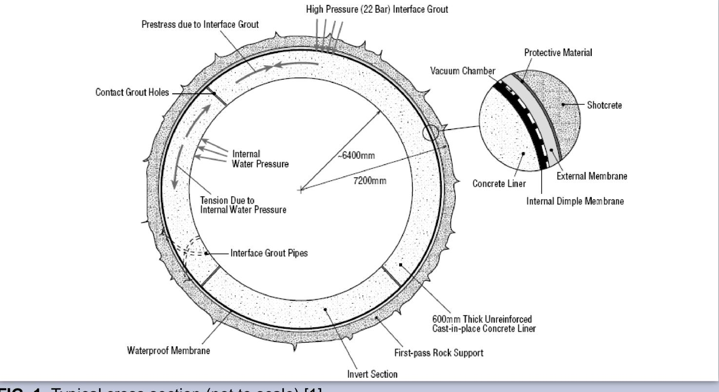
The lining is non-reinforced. Pre-stressing prevents cracking under internal pressures during operation over the entire design life.
