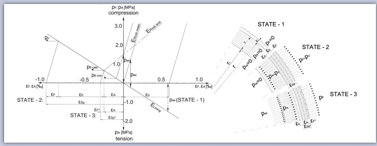
**FIG. 2.** Schematic representation of pre-stressing concept: radial pressure vs. radial strain for rock mass and tunnel lining
