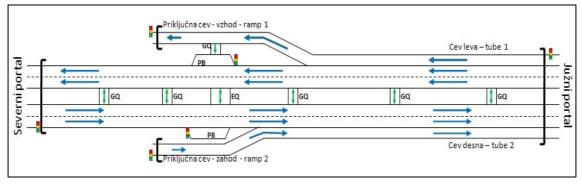
Picture 8: System of tunnel Šentvid with emergency exits
