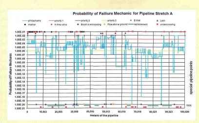
*Figure 3.* Graphic with the result of "Probability of Mechanical Failure" calculation.
