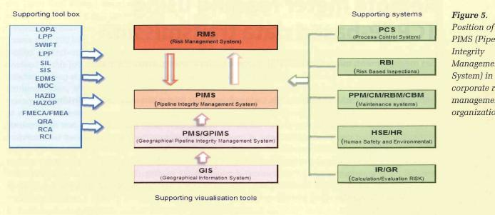
RMS looks at the PIMS, which assesses the integrity of the pipeline installation itself, but also looks at the possible consequences of all pipeline external threats that might cause risks. These risks are not only related to the loss of containment and the costs of repairs or downtime of the pipeline system itself, but are also related to the consequences of an incident to the environment and public safety which could seriously damage the corporate reputation.
