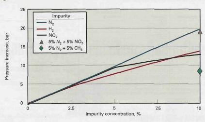
Impurities affect vapor pressure with the exception of  $H_2S$  and  $SO_2$  (Table 4). The values for  $CO_2$ - $SO_2$  mixture are very uncertain, since mixing parameters were estimated and not based on actual measurement data. The presence of impurities also implies the presence of a two-phase region.<sup>3</sup>
