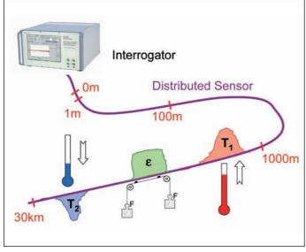
Fig. 2 Brillouin scattering: Temperature and strain profile along optical fiber [8]
