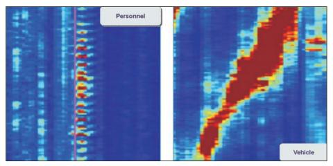
Fig. 4 "Waterfall" diagrams indicating patterns of walking person and SUV [7]
