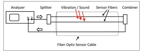
Fig. 3 System block diagram presenting fibre optic interferometer
