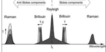
Fia. 1 Scattering effects in fibre optic cables caused by temperature T or strain c [4]
