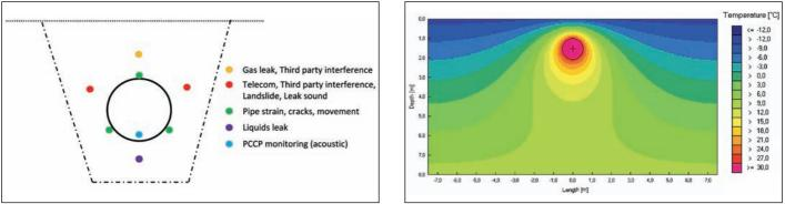
Fig. 5 Application specific sensor location along pipeline
