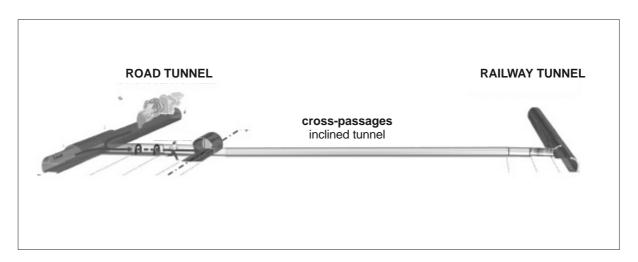
Fig. 3: Cross-passage as inclined tunnel
