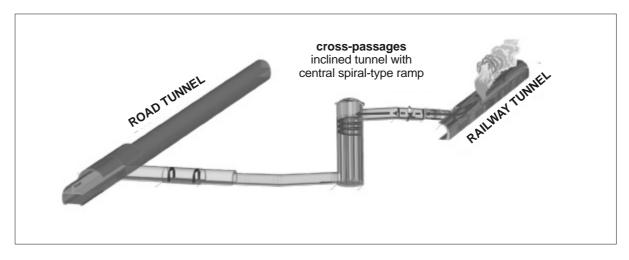
Fig. 4: Cross-passage with spiral-type ramp
