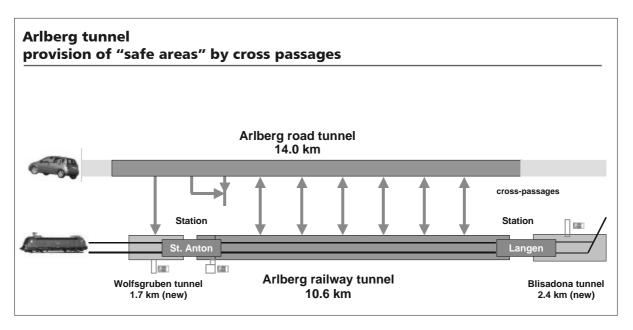
Fig. 2: Arlberg tunnel – Cross-passages between road and railway tunnel
