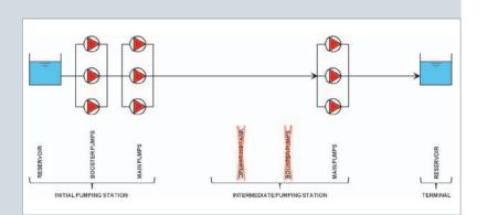
FIGURE 3: Closed pipeline system
