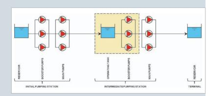
FIGURE 2: Open pipeline system
