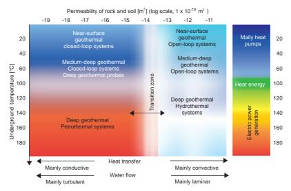
Figure 3.1.7.2: Definition/classification possibilities for geothermal systems based on subsurface permeabilities and depths. | Source: Sass 2012. | Graphic: RENAC.
