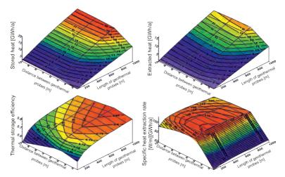
Figure 3.1.7.6: Influence of geothermal probe length and the distances between probes over a range of thermal storage performance indicators, shown for an example system consisting of 37 geothermal probes in 30th year of operation. | Source: Welsch et al., 2015.
