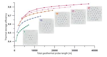
Figure 3.1.7.7: Influence of the number of geothermal probes on thermal storage efficiency, shown for an example geothermal storage system with distances of 5 m between probes in the 30<sup>th</sup> year of operation. | Source: Welsch et al., 2015.
