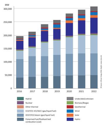
Figure 2.1: Installed capacity by technology type in Africa 2016 – 2022. | Source: African Energy 2018.
