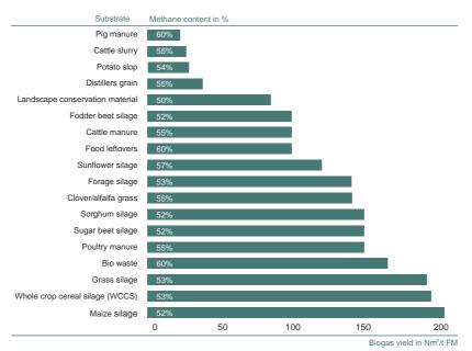
Figure 3.1.5.1: Biogas yield according to substrate in Nm<sup>3</sup>/t FM – FM means 'fresh matter'. | Sources: FNR 2015, KTBL 2015. | Graphic: RENAC.
