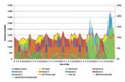
Figure 3.1.9.2.1: Example of hourly simulation results of a hybrid system composed of wind turbines, PV, batteries and diesel gensets. | Source: Lahmeyer.
