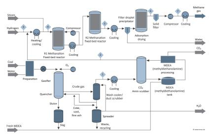
Figure 3.3.4.2.1: Methanation - process diagram. | Source: ILF | Graphic: RENAC.
