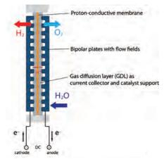
Figure 3.3.4.1.2: Operating principle of a PEM electrolysis cell. | Source: Dr. U.R. Fischer.
