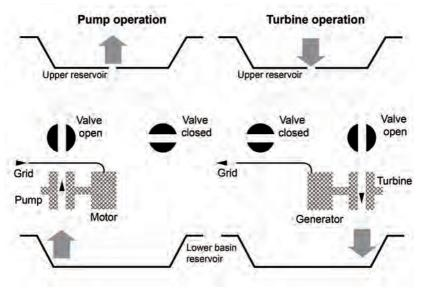
Figure 3.3.1.1.1: Operation of a pumped-storage hydroelectric plant. | Source: Springer Vieweg.
