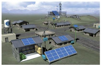
Figure 3.2.1.3.1: Example of a mini-grid with decentralised PV, wind turbines, batteries, a diesel generator and a distributuion grid/network. | Source: http://www.ennera.com/en/detail-solution/minigrids.
