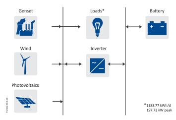
Figure 3.1.9.2.2: Example of the schematic modelling of a hybrid system. | Graphic: RENAC.
