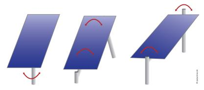
Figure 3.1.3.3: Single-axis tracking PV module mounting system. | Source: RENAC.
