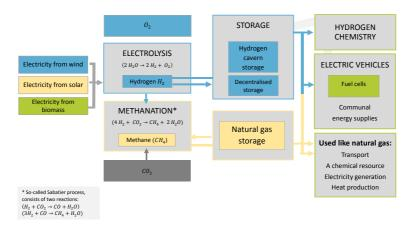
Figure 3.3.5.1: The hydrogen added value chain. | Source: HYPOS.
