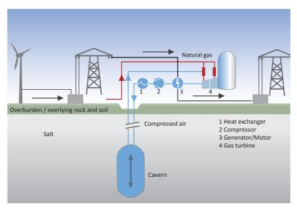
$\label{eq:Figure 3.3.1.3.1: Schematic of a diabatic CAES (compressed air energy storage) power plant. | Graphic: RENAC.$
