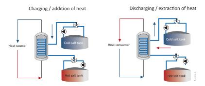
Figure 3.3.2.2: Operating principle of a thermal salt storage system. | Graphic: RENAC.
